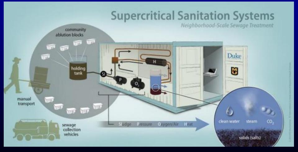
In supercritical water, organics are rapidly oxidized (in seconds) resulting in heat, and CO<sub>2</sub>
